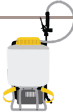
Backpack sprayer - 4 gallons to 4 1/2 gallons either pump or electric and paint screen for screening release into sprayer
